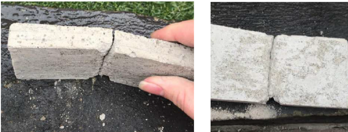
Photo 7. Failure with rebar. (Student: Aranza Valentina Barragán, Nov 2020)
