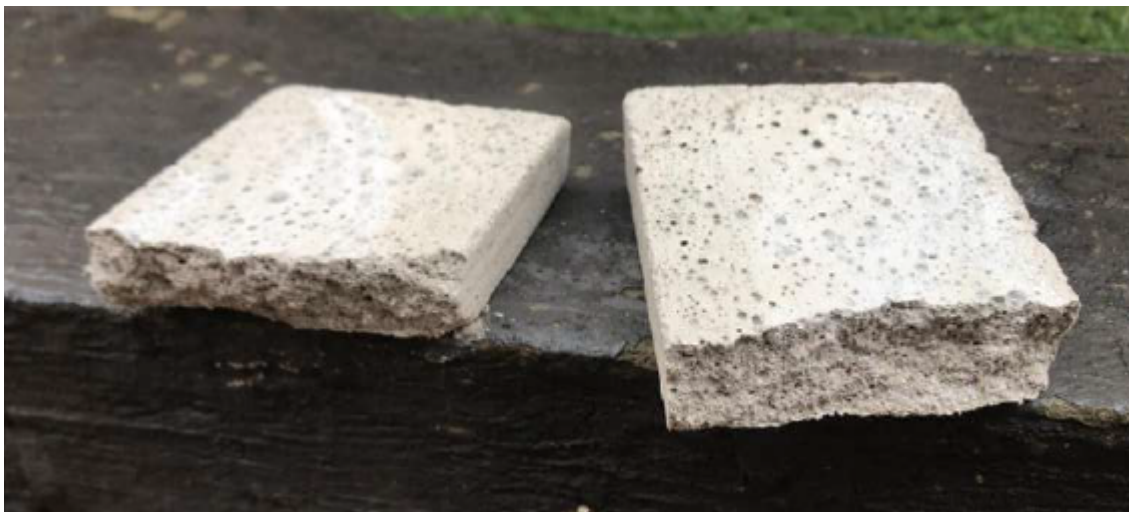
Photo 6. Failure without rebar. (Student: Aranza Valentina Barragán, Nov 2020)
